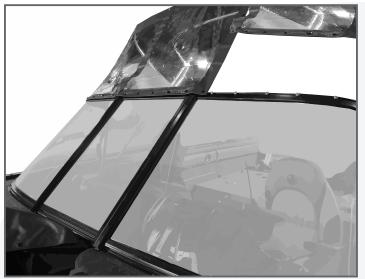
Repeat adding Screw Studs and snapping into place until the Front Windscreen and Door are installed.
