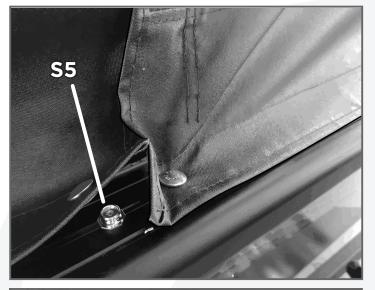
Using a 9/64" drill bit, drill a pilot hole and install the Pull-the-Dot Screw Stud (S5) into the Gunnel.
