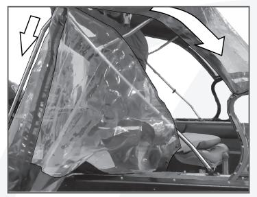
Zip the Port, Starboard and Rear curtains onto the Bimini Frame.
