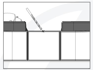
Using a \*pontoon rail specific\* drill bit, drill a pilot hole into the front of the Railing, do not drill through both sides.
