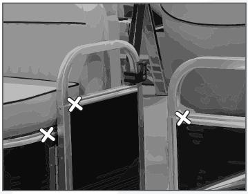
Navigate to the Stern of the Boat and mark the mounting locations of any sharp corners onto the Cover and Railing.
