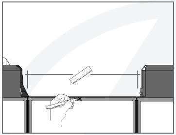
Measure the door opening at the Bow and mark the center location for the Screw Stud onto the Door Rail.
