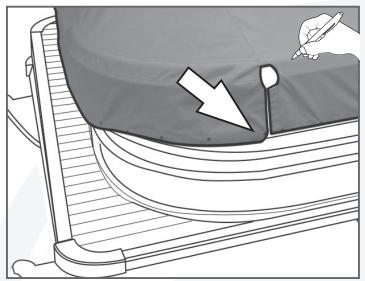
Locate the nearest Velcro on the Side of the Pontoon near the Bow, pull the Cover taut and mark the Snap location onto the Cover.
